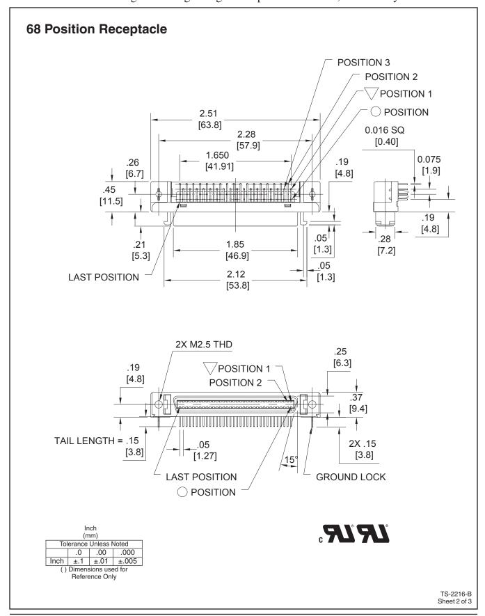
.050" Boardmount Through-Hole Right Angle Receptacle - Shielded, SCSI-2 Layout
